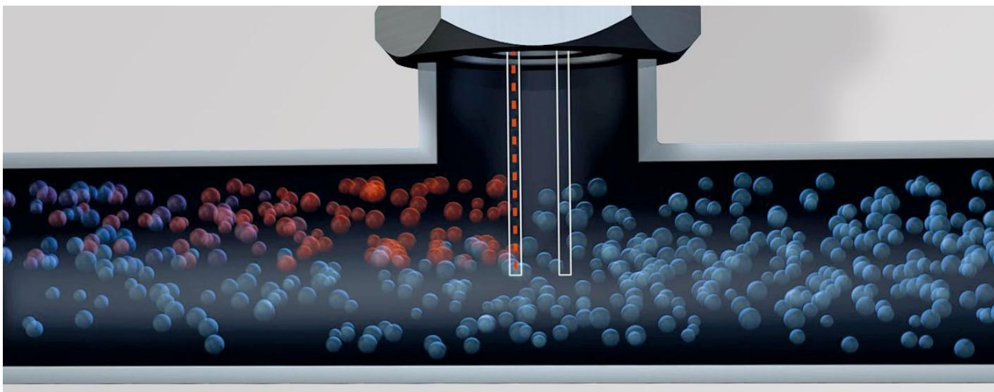
Two temperature sensors are installed in series in the direction of flow. The first temperature sensor measures the current process temperature of the compressed air, while the second sensor is electrically heated to a temperature that is 40 K higher than that of the first sensor.
