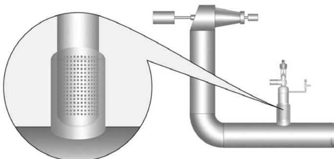
Dump tube installation for Air Cooled Condenser
