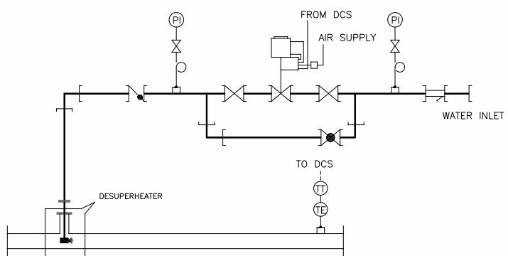
CIR 3530 PRDS station includes a pressure and temperature control loop and is used to condition the steam generated from the boiler to the desired outlet pressure and temperature. Main components of Pressure control loop are CIR 3100 or CIR 3400 steam pressure valve & bypass arrangement along with pressure transmitter(PT) and local gauges which aids in controlling the steam pressure suitable to process requirements.
