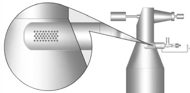
Dump tube installation for Water Cooled Condenser
