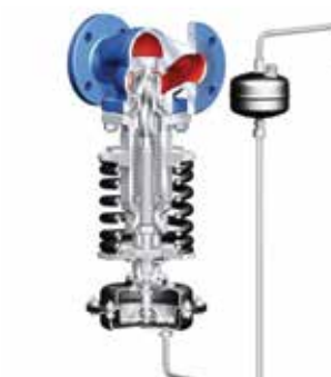
Pressure Reducing Valve
