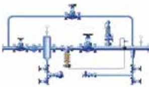
Pressure Reducing Station
